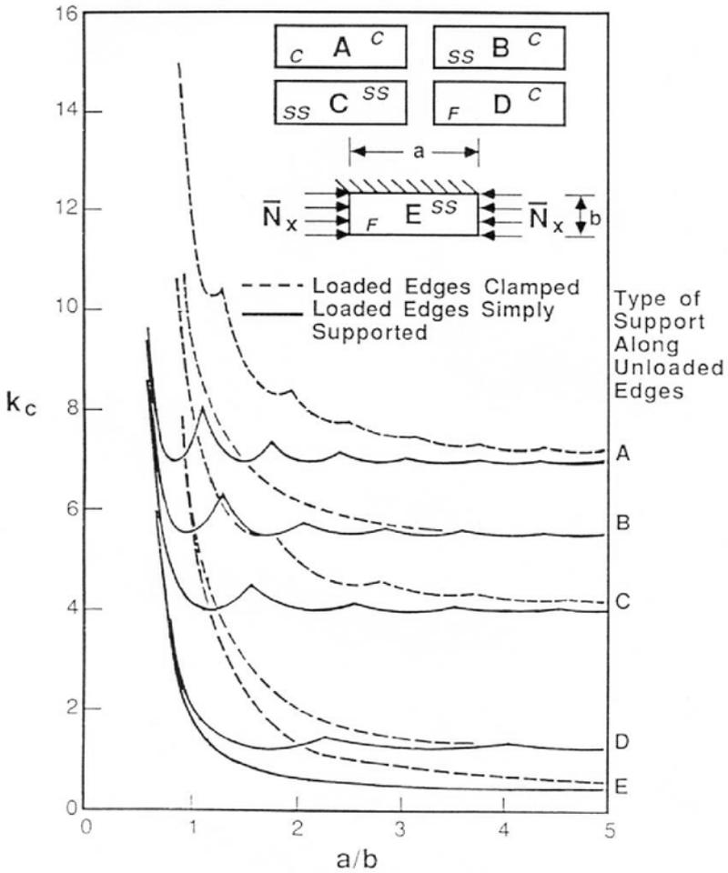
Figure 6.8. Compressive-buckling coefficients for flat rectangular isotropic plates.
