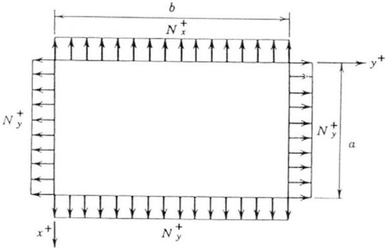
Figure 6.4. Rectangular plate subjected to in-plane loads.
