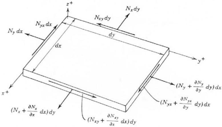
Figure 6.1. In-plane forces on a plate element.
