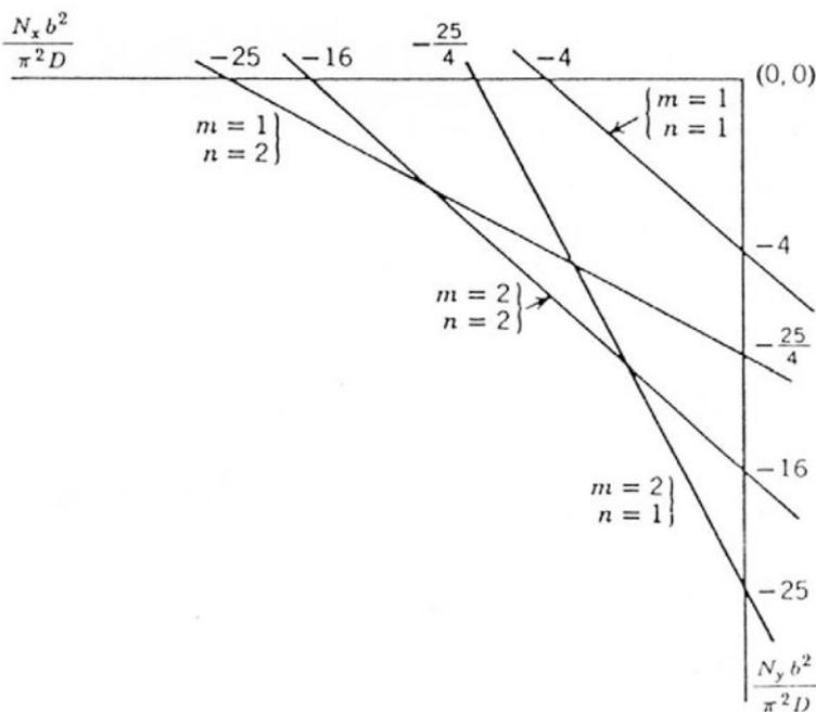
Figure 6.5. Values of biaxial loads causing buckling for square simply supported isotropic plate.
