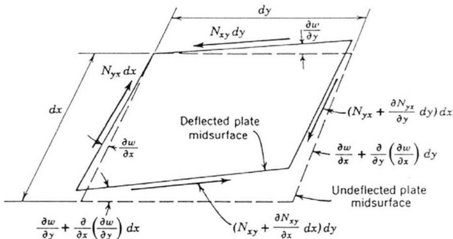
Figure 6.3. In-plane shear forces acting on a deflected plate element.
